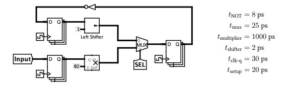
The left shifter combinational logic block shifts the top input by the number of bits indicated by the bottom input. The shifter in the diagram shifts the output of the connected register left by 1 bit.
