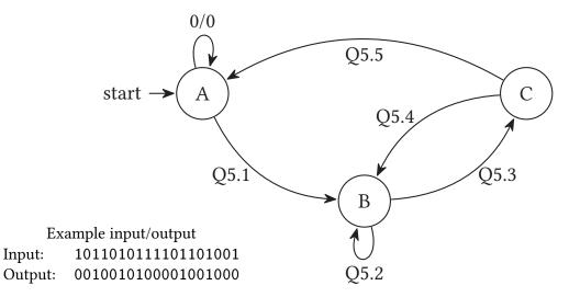
For each of the transitions above, fill in the appropriate input and output values such that the FSM behaves as described.
